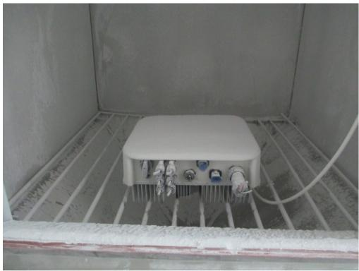
Test setup of IP6X
